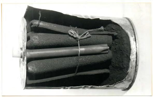
the filter unit was installed. This break-in period provided adequate distribution of the carbon charge on the septum. The precoated septum is shown in Figure 8.
